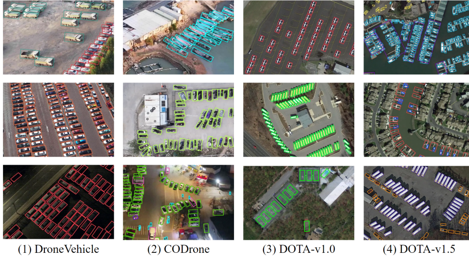
Fig. 1: The illustration of the placement prior in representative UAV and remote sensing datasets. Generally, the target objects are placed on the ground plane in a context, rather than exhibiting arbitrary distribution.
