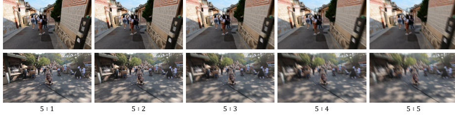
Fig. 5: Example frames from our REDS-ME dataset across five exposure levels and two scenes. Each column corresponds to an exposure ratio from 5:1 (shortest exposure) to 5:5 (longest exposure). Longer exposures lead to increasingly severe motion blur, illustrating the controlled effect of exposure variation on blur extent.
