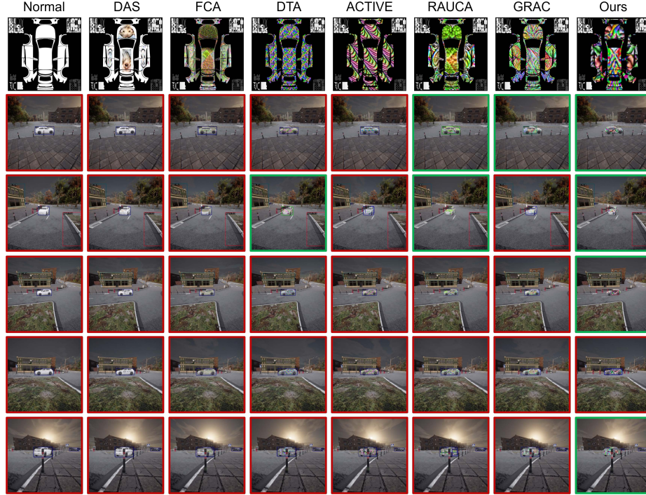
Fig. 4: Qualitative evaluation in the digital environment. The top row compares the optimized 2D textures. The subsequent rows display rendering results under varying distances, camera angles. Green image borders indicate successful evasion, while red borders denote detection failures.
