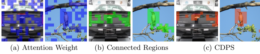
Fig. 3: Visualization of selected patches in each step. We illustrate the selection process using two examples: (a) initial patches selected by attention map (blue); (b) extraction of the connected regions (green) to isolated patches; (c) the final discriminative patches (red) to construct CDPS.
