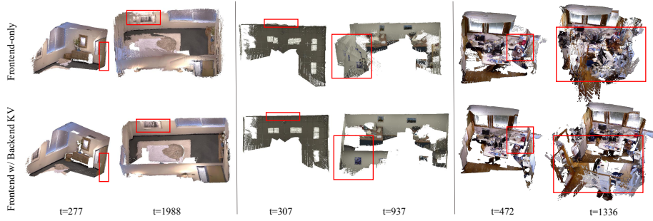
Fig. 5: Qualitative reconstruction comparison with and without backend assistance. The first row displays the frontend-only results at the corresponding timestamps, while the second row shows the results with the assistance of backend KV caches.
