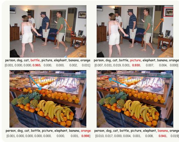
Fig. 4: RoI Align on feature regions. We map the bounding boxes to the feature map of the image and perform RoI Align accordingly, then compare the extracted features with the output embeddings of the text encoder for classification. RoI Align effectively preserves the VLM’s generalization capability for classification.
