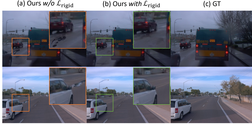
Fig. 4: Enforcing rigid regularization ( \mathcal{L}_{\text{rigid}} ) removes the structural floaters seen around rigid objects in (a).
