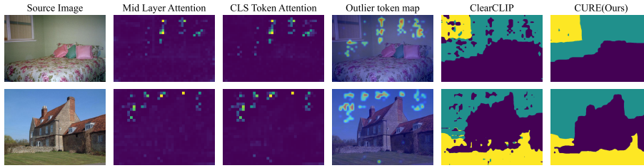
Fig. 1: Visualization of token attention patterns and segmentation outputs. The second column shows the average attention map across all tokens from an intermediate layer, revealing global context entanglement. The third column visualizes the final-layer CLS token attention, which encodes aggregated global information. The fourth column presents a norm-based heatmap highlighting outlier tokens that exhibit global attention artifacts. The fifth and sixth columns compare the segmentation results of ClearCLIP [22] with the refined outputs produced by our proposed method, CURE.
