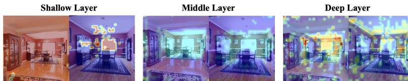
Fig. 6: Region-wise Anchor Depth Importance. In the middle layer, the importance of depth anchors is highly related to the actual depth, while this correlation is not significant in both the shallow and deep layers.
