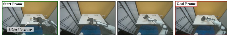
Fig. 10: Real Robot Example. Given goal and start images, DexWM successfully plans and executes the trajectory by finding the optimal actions using the Cross-Entropy Method. Notably, DexWM works zero-shot without any real-robot training.
