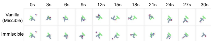
Fig. 7: Immiscible diffusion boosts the performance of diffusion policy. The robot (circle) needs to push the T-shaped object (gray) into the desired place (green).
