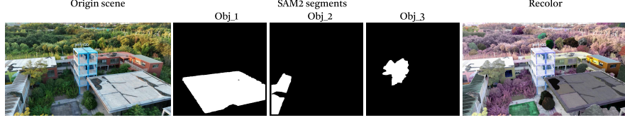
Fig. 3: Example of SAM2-based recoloring. Starting from the original scene (left), SAM2 produces object masks (middle), which are then used to apply recoloring to selected regions, yielding the recolored result (right).
