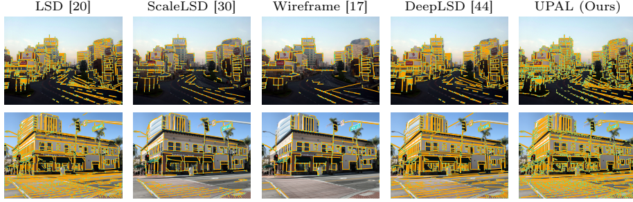
Fig. 4: Line detection examples. In spite of its efficiency, UPAL outputs generic lines with quality similar to more expensive methods.
