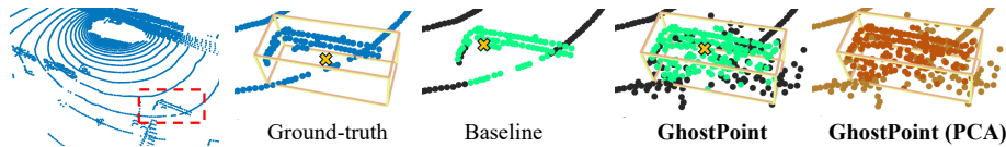
Fig. 1: GhostPoint learns beyond visible LiDAR surfaces. Raw scans observe only sparse object returns, causing discovered pseudo-instance centers to be biased toward visible surfaces. From these pseudo instances, GhostPoint samples adjacent unobserved regions and hallucinates their latent representations, producing features whose centers better align with the ground-truth object centers, marked by yellow crosses, while recovering object-level structure as illustrated by the PCA visualization.
