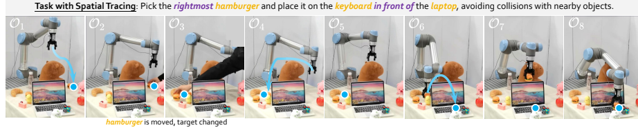
Fig. 5: Real-World Evaluation. The blue trace denotes predicted spatial trace in 2D, and the blue dot marks current target. RoboTracer can generate spatial traces whose start and end points all satisfy spatial constraints in cluttered and dynamic scenes.
