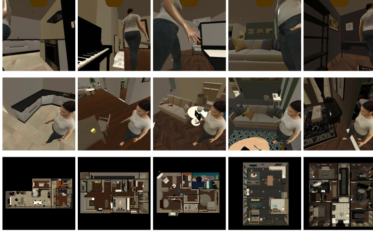
Fig. 2: Visual examples of the CoT-HRC benchmark across diverse simulated indoor environments. For each task scenario, we synchronously capture video streams from three perspectives: the constrained 0.4m robot egocentric view (Top row), the unobstructed third-person tracking view (Middle row), and the global top-down view (Bottom row). Compared to the ideal perspectives, the egocentric view inherently suffers from severe field-of-view truncation and dynamic torso occlusions, highlighting the realistic perception challenges.
