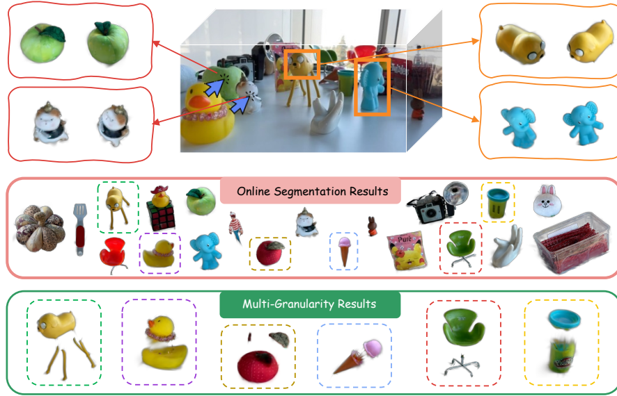
Fig. 5: Online segmentation results of SAGO on the Figurines scene. The granularity is simply determined by the initial mask obtained via SAM prompted by the user, and the segmentation is iteratively refined through NBV-based online updates.
