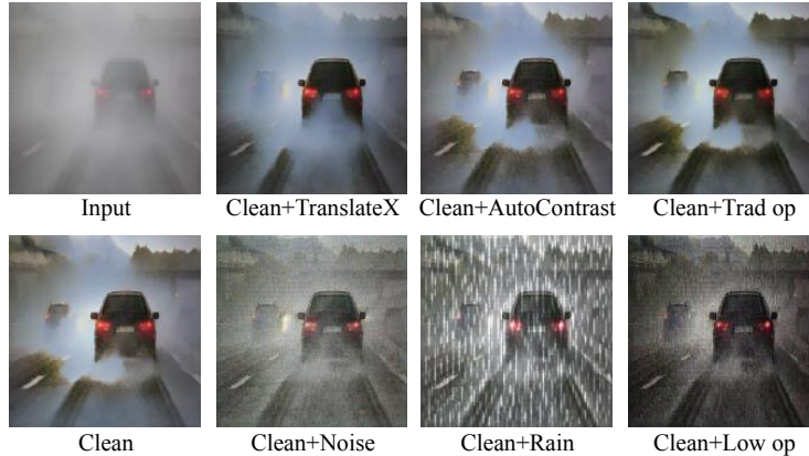
Fig. 4: Low-level degradations induce stronger surface-statistical shortcuts while preserving image clarity than traditional augmentations. We compare different augmentation strategies applied to target-domain clear images. Traditional augmentations introduce only weak surface-statistical changes, which may still allow semantic hallucinations. In contrast, explicit low-level degradations create stronger low-level variations and encourage the discriminator to focus on degradation-related cues. Despite these injected degradations, the images largely preserve the underlying characteristics of the clear domain.
