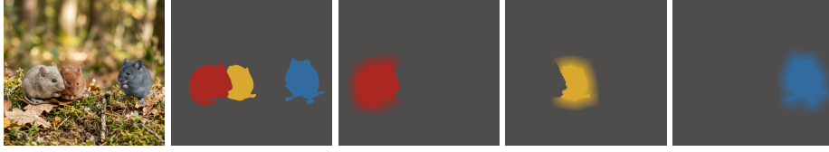
Fig. 2: Instance-aware smoothing strategy. Each segmentation mask is smoothed independently, and the smoothed values are zeroed when touching the edge of a neighboring, non-smoothed mask ( e.g. , the red and yellow masks). If an instance is sufficiently distant from the others, its mask is smoothed with no constraints ( e.g. , the blue mask).
