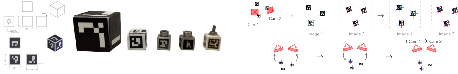
Fig. 4: Left: ArUco calibration cube design iterations leading to our final 8 mm wooden cube design. Right: ArUco-based pose estimation pipeline: (1) marker detection, (2) PnP pose estimation, (3) relative transformation via RANSAC and refinement.
