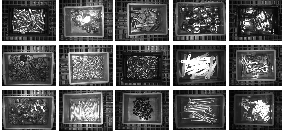
Fig. 1: XYZ-IBD is an industrial-grade dataset for object detection and 6D pose estimation, providing sub-millimeter annotation precision for reliable evaluation. Unlike household datasets, XYZ-IBD focuses on the perception bottleneck of robotic manipulation: tackling multi-instance ambiguity, randomly stacked scenarios, heavy occlusion, geometric symmetries, and extreme specular reflections. We benchmark the recent SOTA object detection and pose estimation under both object-specific and unseen-object setups, revealing a significant performance gap, challenging existing SOTA methods to bridge the divide between laboratory benchmarks and real-world factory complexity.
