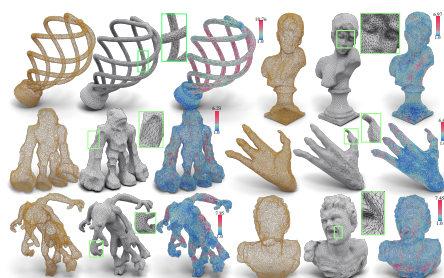
Fig. 5: Our anisotropic surface mesh approximation from input point clouds. The models are selected from Thingi10K dataset [73]. Left to right: input point clouds, reconstructed anisotropic meshes with zoom-in views, and estimated curvature tensors with stretching ratios for input point clouds in colors.
