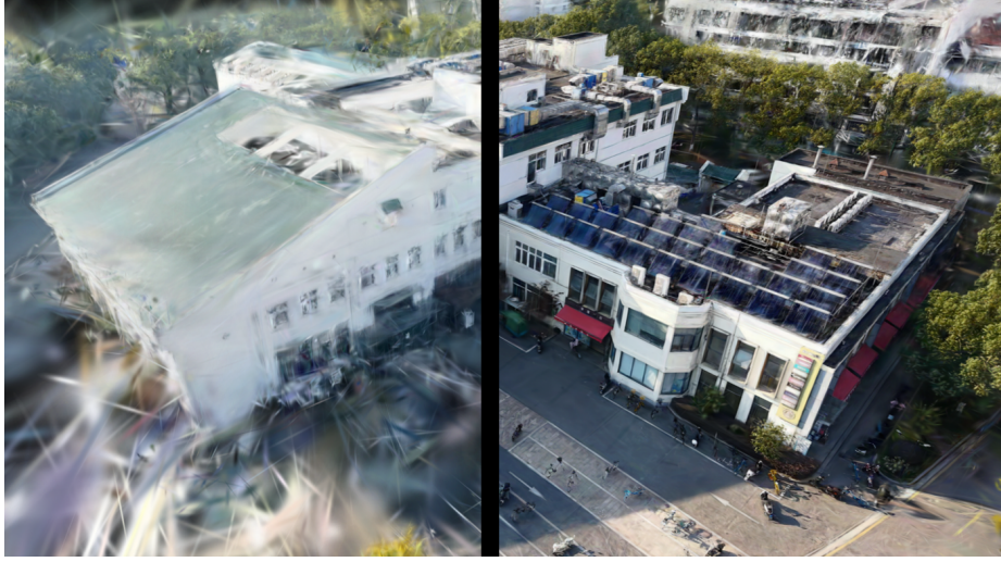
Fig. 4: Outlook: Real-World Campus Digital Twin Maintenance. Flash-Refine deployed on a custom drone-captured campus dataset. When a specific building suffers from texture degradation or missing geometry due to initial flight path limitations, a brief supplementary drone flight allows our method to seamlessly inject the missing high-frequency architectural details directly into the massive city-scale “ply” asset within minutes.
