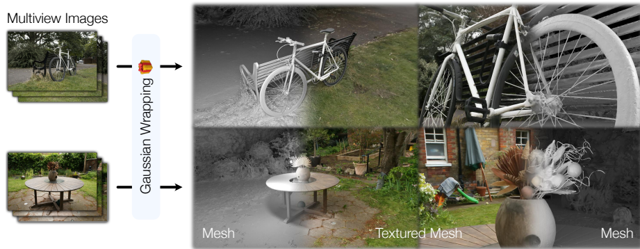
Fig. 1: High-fidelity surface reconstruction from 3D Gaussian Splatting. Our method, Gaussian Wrapping, reconstructs watertight and textured surface meshes of full 3D scenes given multiview RGB images, by interpreting 3D Gaussians as stochastic oriented surface elements. This figure illustrates the resulting surface meshes, with and without the RGB texture. Our meshes represent the full scene—including background geometry and extremely thin structures such as bicycle spokes where existing methods fail—with a significantly more compact representation than concurrent works [9, 56].
