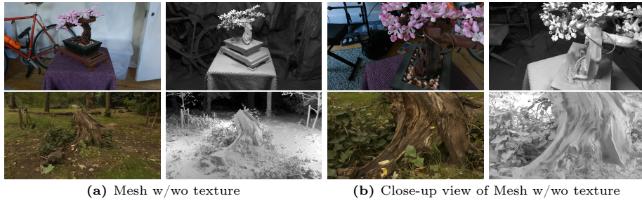
Fig. 2: Examples of textured meshes reconstructed with our method. While being watertight and lighter than meshes reconstructed by state-of-the-art methods, our approach is able to reconstruct extremely fine details such as a few blades of grass—as can be seen in the close-up view of the stump scene [5].
