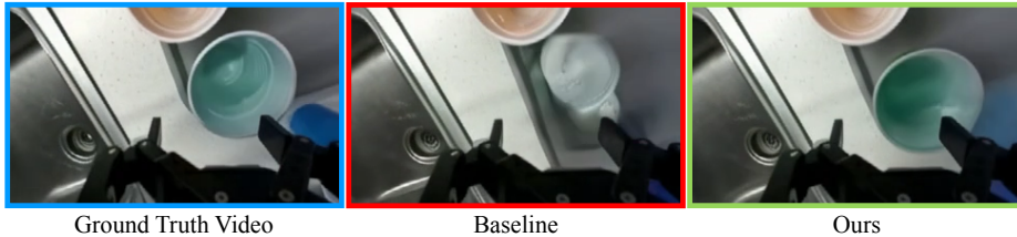
Fig. 1: Autoregressive video rollout quality. We use an action-conditioned robot world model to generate multi-view image predictions from a single observed state. The ground-truth (blue) is compared against the baseline (red) and our post-trained model PersistWorld (green). While the baseline accumulates error and destroys the object (cyan bowl) within seconds, our method maintains structural integrity and spatial consistency, establishing a new state-of-the-art in rollout fidelity.
