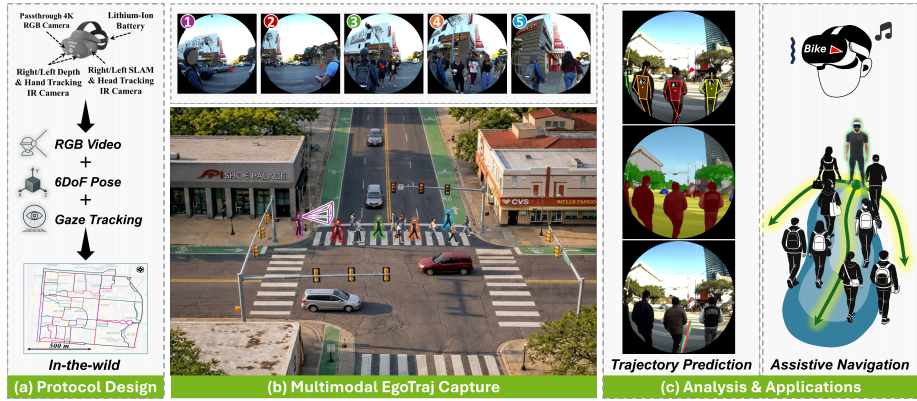
Fig. 1: Overview of EgoTraj. (a) Protocol design: the Meta Quest Pro headset records synchronized 6DoF head pose, gaze signals, and egocentric RGB video during real-world outdoor navigation. (b) Multimodal EgoTraj capture: representative egocentric frames from a crosswalk navigation scenario with multiple social interactions. (c) Analysis and applications: the dataset supports downstream tasks such as assistive navigation for blind and visually impaired users.
