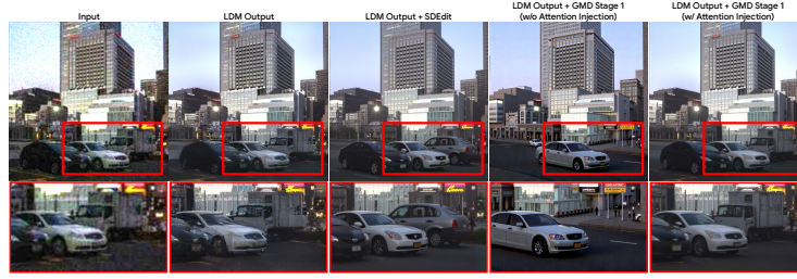
Fig. 8: Visual comparison of pseudo-target generation strategies (Stage 1). We evaluate the intrinsic quality of different generation methods. Standard baselines like SDEdit [32] or the flow matching inversion without Attention Injection help remove artifacts but suffer from severe content drift and structural distortion (e.g., altering vehicle geometry). In contrast, our adopted method with Attention Injection effectively restores details while strictly preserving the original structural layout.
