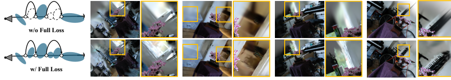
Fig. 8: Comparison of novel-view renderings with/without the Full Loss. We use a pre-selected view order from FisherRF † to ignore view-selection effects. The w/o Full Loss ( \mathcal{L}_{sub} only) variant exhibits smoothing artifacts, whereas w/ Full Loss ( \mathcal{L}_{full} + \mathcal{L}_{sub} ) preserves scene structure and high-frequency details.
