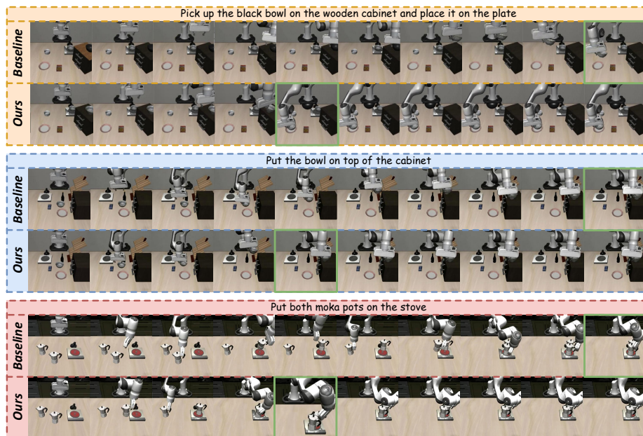
Fig. 3: Qualitative comparison on randomly sampled LIBERO tasks. Under identical configurations, the baseline incurs redundant physical actions, whereas PolicyTrim achieves task completion in roughly half the steps.
