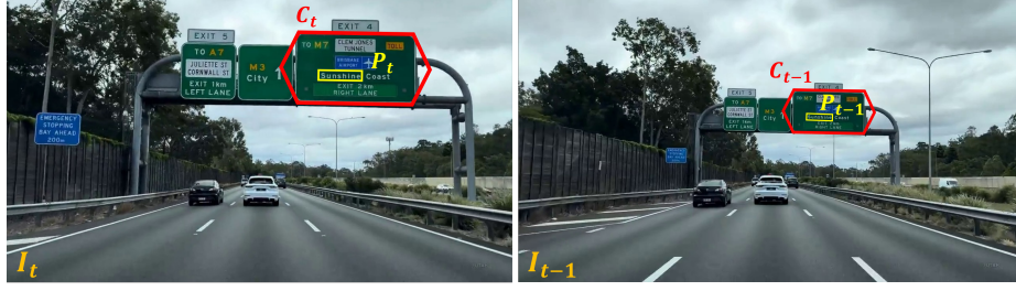
Fig. 2: Geometric correspondence through core polygon at frame t (left) and t-1 (right) in case n=6 . The mapping \mathbf{H} between core polygons C_t and C_{t-1} is used to project the detected text region P_t back to its position in the previous frame P_{t-1} .
