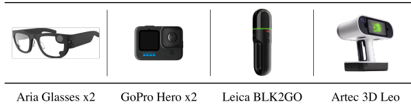
Fig. 8: Sensors used to create the CoMind dataset. Two Aria glasses record the scene from each participant’s view. Two GoPro Hero cameras capture exocentric views. The Leica BLK2Go and Artec 3D Leo are used for 3D scene and object scanning respectively.
