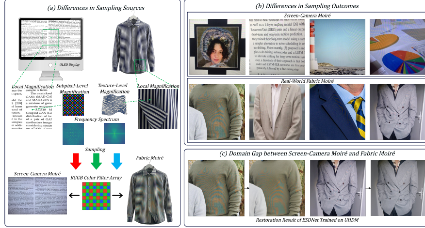
Fig. 1: Cause-to-appearance domain gap between screen moiré and fabric moiré. (a) Sampling sources: screen moiré originates from rigid planar displays with regular pixel/subpixel lattices, while fabric moiré arises on non-rigid, deformable garments with anisotropic weave microstructures, undergoing folds, stretching, and pose variations. (b) Sampling outcomes: screen moiré is typically global and content-agnostic, whereas fabric moiré is localized to high-frequency textile regions and strongly coupled with texture and deformation. (c) Domain gap: these differences hinder transferring screen-trained models, leading to moiré residual or over-smoothing.
