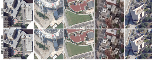
Fig. 5: Render refinement. (a) Original 3DGS render with artifacts and blurry textures; (b) Refined result showing enhanced geometry and texture quality.
