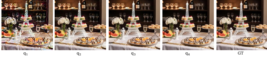
Fig. 3: An example of Hierarchical Binary Quantization ( M=4 ). For q_1 , q_2 , and q_3 , we truncate the complete sequence and take the truncated parts for reconstruction.
