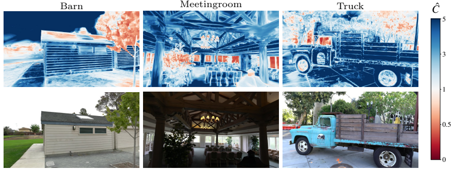
Fig. 3: Confidence-Driven Gaussian Splatting: We show rendered images from our trained method, accompanied by the rendered confidence maps \hat{C} . The confidence maps effectively isolate reflective surfaces, thin foliage, or rarely observed areas (such as the roof for Barn). Importantly, the low-confidence regions are still well-reconstructed.
