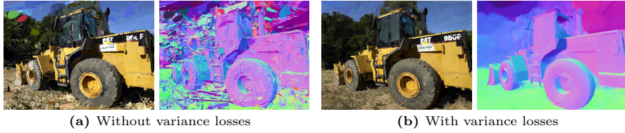
Fig. 4: Effect of our proposed Variance Losses: Rendering color and normals only for the first-hit Gaussians shows how the variance losses align individual Gaussians better to the true object surface, in both color and orientation.
