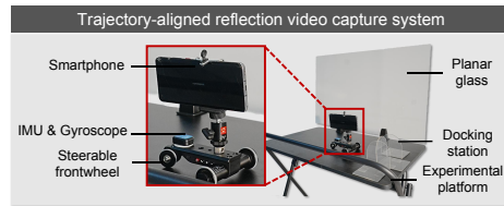
Fig. 3: Trajectory-aligned video capture system for DUALREF-V. A programmable dolly ensures reproducible camera trajectories. It captures paired mixture and transmission-only ground truth by repeating paths with and without a removable glass panel, while an IMU & Gyroscope module records motion data.
