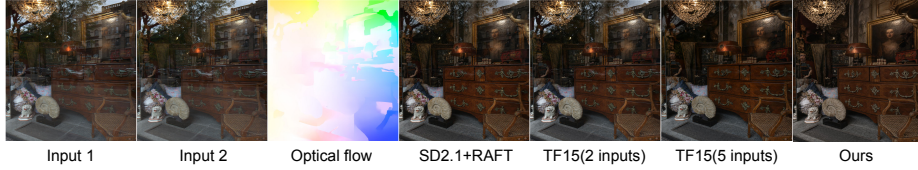
Fig. 8: Analysis of explicit flow on the Burst dataset [9]. We compare against the SD2.1+RAFT and TF15 [81] baseline with different number of input frames. Explicit flow becomes unreliable in reflection-corrupted regions and needs more frames to reduce ambiguity, whereas our method produces robust results from only two views.
