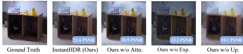
Fig. 7: Ablation visualization. Attn.=cross-view attention, Exp.=exposure normalization, Up.=upsampling. Removing Attn. causes wall ghosting; removing Exp. shifts overall brightness; removing Up. produces blurry results.
