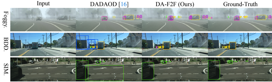
Fig. 4: Qualitative comparison between DADAOD [16] and the proposed DA-F2F across three adaptation scenarios. From the first to fourth columns: input images, detection results of DADAOD and DA-F2F, and the ground-truth annotations.
