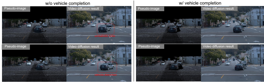
Fig. 7: Ablation study on vehicle completion. Vehicle completion fills in unobserved surfaces in the pseudo-images, effectively eliminating vehicle distortion and texture artifacts in the diffusion outputs.
