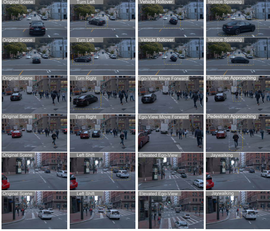
Fig. 3: Qualitative demonstrations of ReinDriveGen on OOD safety-critical corner cases. Every two consecutive rows show two frames from the same scene, with the edit type and edited region annotated in each image.
