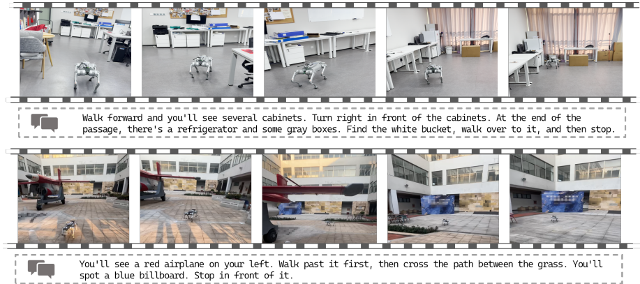
Fig. 4: Navigation results in real-world indoor and outdoor environments. Experimental results demonstrate that, regardless of whether the agent is navigating through complex, confined indoor spaces or outdoor scenarios with challenging illumination conditions, the proposed model consistently and accurately comprehends natural language instructions, enabling it to rapidly plan and execute precise navigation trajectories.
