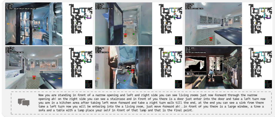
Fig. 3: Visualization of AgentVLN’s navigation. Green points represent the visual prompts generated by the perception-level skills, whereas red circles denote the navigation waypoints selected or predicted by the model. Notably, when traversing narrow passages or confronting severe visual occlusions, the model seamlessly outputs fine-grained atomic actions for trajectory fine-tuning. This demonstrates its robust capability to achieve highly accurate, collision-free navigation relying exclusively on egocentric observations.
