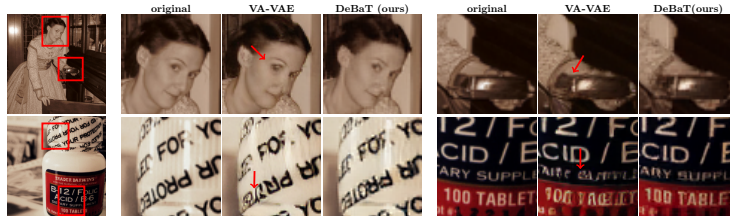
Fig. 1: Reconstruction quality for two examples. We compare the reconstruction of VA-VAE to our approach DeBaT. Highlighted regions emphasize textures and edges. DeBaT better preserves high-frequency details and sharp structures, producing reconstructions visually closer to the input. Arrows indicate reconstruction errors.
