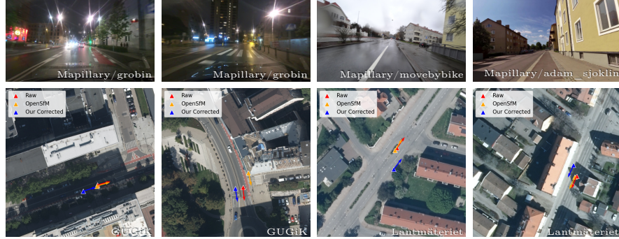
Fig. 7: Visual comparisons of the different pose annotations available for Mapillary images in our OpenCVL evaluation. The corrected Mapillary pose is significantly better than the raw Mapillary GNSS tag and the Mapillary-reported OpenSfM corrected pose.
