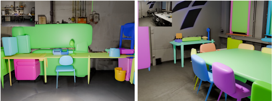
Fig. 7: Robustness on real-world point clouds. We show results from two ScanNet++ scenes where objects are decomposed into sets of superquadrics by our robust SuperFlex variant. Different colors indicate different object instances. A rendering of the original scene is shown in the top-left corner.
