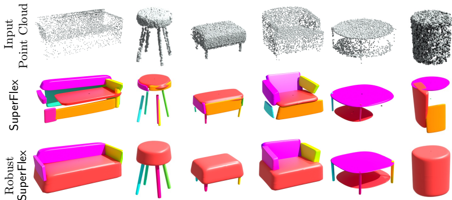
Fig. 6: Qualitative Results on ASE. Top row: partial input point clouds. Below: the outputs of our standard SuperFlex and its robust fine-tuned variant.
