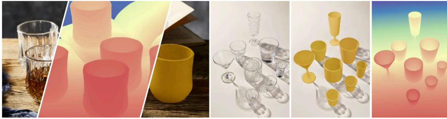
Fig. 1: SeeClear is a novel framework that converts transparent objects into diffusion-generated opaque images, predicting stable and accurate depth for transparent objects.
