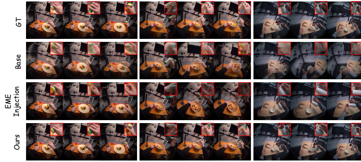
Fig. 5: Qualitative results for ablation of ego-motion consistency Rows: GT, Base, EME Injection, Ours (EgoHOI). EME mitigates long-horizon ego-motion drift and improves viewpoint stability. Zoom-ins highlight cleaner details under viewpoint changes. The full model best matches ATE/RRE/RPE gains.
