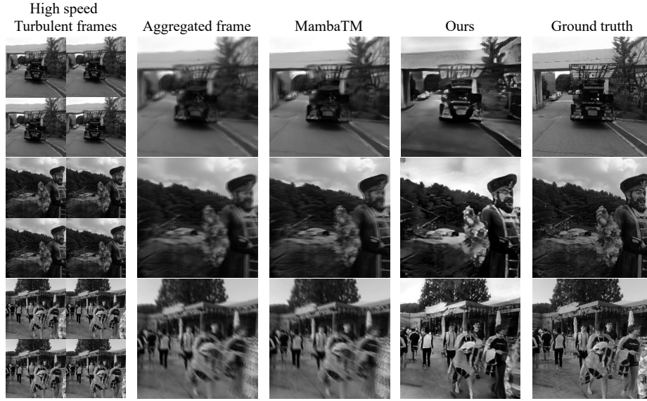
Fig. 8: Simulated high-speed scenes show that event light fields recover sharper images than frame-based methods. Motion-blur cannot be compensated for by frame-based methods, which occurs when scene dynamics or turbulence are fast. Event-based light fields operate directly on the event stream and reconstruct the underlying scene without blur caused by integration. Motion-blur is simulated by aggregating 4 conventional frames into a single blurred frame.
