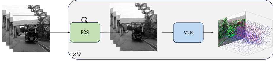
Fig. 4: Simulation pipeline. Turbulence is added to clean frames using a turbulence simulator based on the phase-to-space (P2S) transform [33]. V2E converts turbulent frames to events [20]. The process is repeated 9 times to simulate a 3 \times 3 light field. The network is trained on simulated data and generalizes to tabletop experimental settings.
