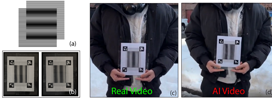
Fig. 1: (a) The Moiré effect, created by overlaying two repetitive layers. (b) Our prototype Moiré signature assembly. Viewing the assembly from slightly different camera angles (left vs. right) causes the fringes to shift in phase according to deterministic physical laws. (c) In a real video, Moiré fringes appear naturally and shift predictably with camera movement. (d) In an AI-generated video, the fringes distort, and their phase shifts do not adhere to the underlying physics.
