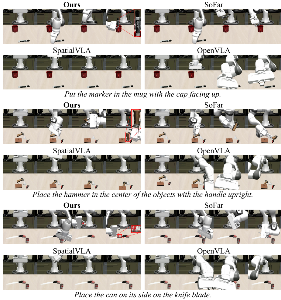
Fig. 4: Qualitative Comparison on Robot Manipulation Using Open6DOR V2 Objects and Scenes. Our method predicts both position and orientation more accurately than the baselines.
