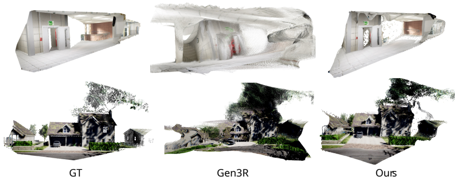
Fig. 4: Point cloud forecasting on TartanAir. Gen3R produces structurally disorganized geometry on walls and rooftops, whereas our method preserves coherent structure and yields more accurate predictions.
