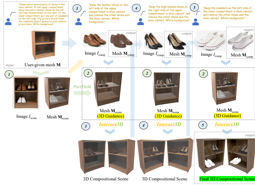
Fig. 6: More than two parts composition results. Given a cabinet mesh, we render an image from it, add three pairs of shoes to the image using Nano Banana Pro and generate it with TRELIS2 to obtain the object-object spatial relationships (OOR). Next, we use Nano Banana Pro again to extract each individual object in the shoe cabinet and generate them with TRELIS2. Finally, using the OOR information, we sequentially add them to the cabinet mesh to form an interactive 3D scene.
